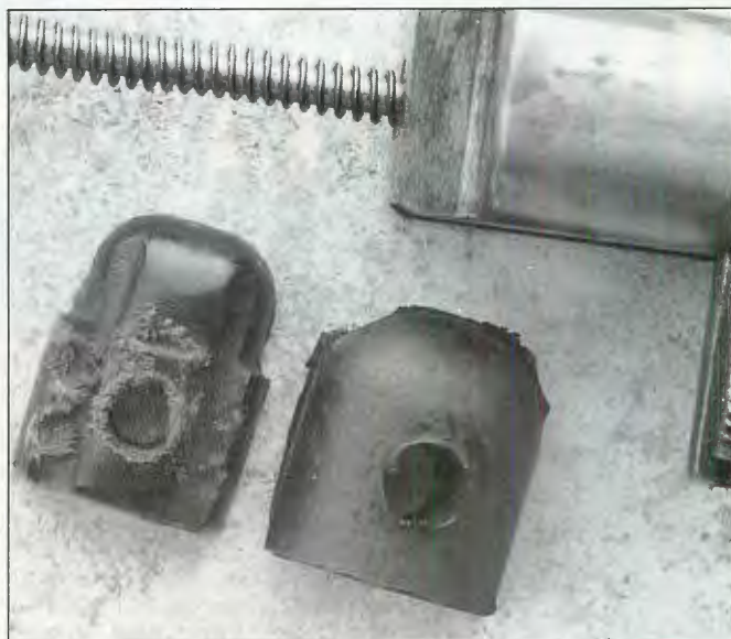
Russian fiber buffer on the left is longer than the Chinese Type 50 rubber buffer and cannot be used in the Type 50 without modification.
